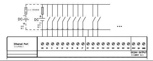
◆ 因为公共端 CO/C1/C2 彼此独立,使用相同输入类型时,请使用短接线将公共端连接。As the common terminals CO/C1/C2 are independent of each other, when using the same type of input, please connect the common terminals using short wires.
