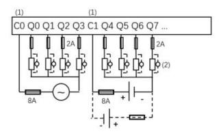
CO和C1端子未在内部连接。CO and C1 terminals are not connected internally.
